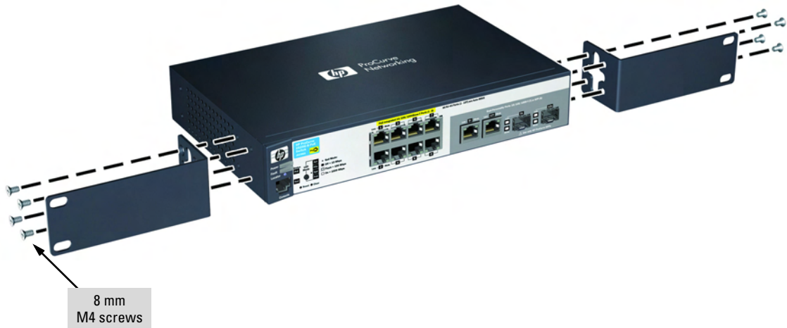
Figure 2-5. Attaching mounting brackets
